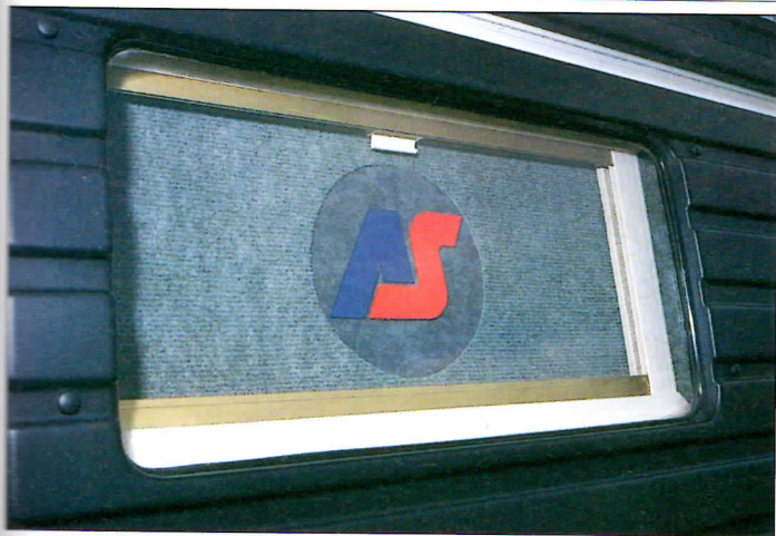
Cassette blinds are prone to damage, and not always effective. "They're a curse," says Bill. These removable boards overcome the problem completely, and have a dedicated stowage spot behind the wardrobe door.
