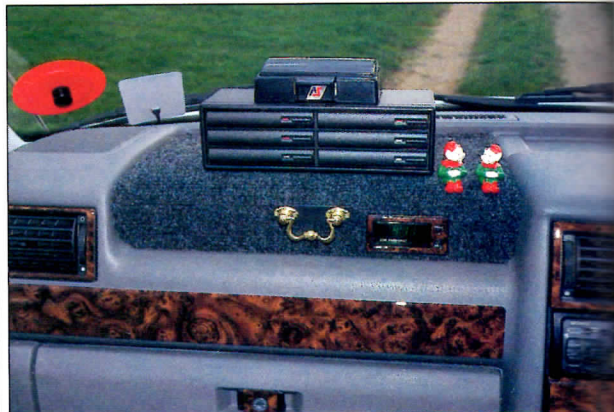
Bill hasn't been able to resist adding a few extra gizmos to the dashboard, including that wood-rimmed steering wheel. Note the cup holder on the door armrest. Additional instrumentation includes altimeter, compass and landmeter. Lid cover makes good use of the otherwise useless scooped-out section of dashboard in front of the passenger. The box on top takes cassette tapes.
